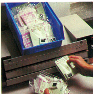
10: Each component, along with a descriptive packing label, is sealed in a plastic bag.
