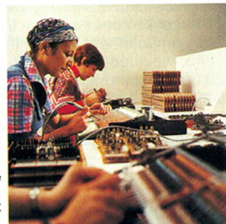
16: All WERSI products are also available fully assembled. Here the components are put into the circuit boards.
