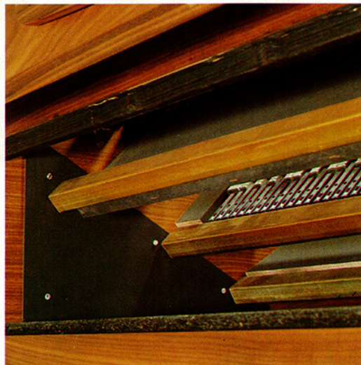
Novel Hinge System for manuals and stop board. Patent pending.
